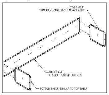
**Step 2:** Turn the back panel on its back with the shelves pointing upward. Attach the first side panel, the left rear leg, and three compartment dividers to the assembly from Step 1.
