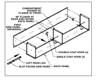
Step 3: Attach the second top shelf, the second bottom shelf, and an additional two single coat hooks to the second back panel as in step 1.
