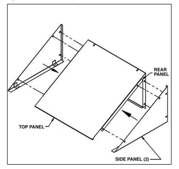
Step 3: Attach the sloping hood to the top of the locker with slotted #8 - 32 screws (provided).
