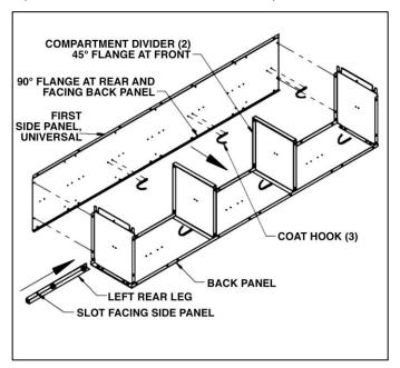
**Step 3:** Attach the second top shelf, the second bottom shelf, and an additional three coat hooks to the second back panel as in step 1.
