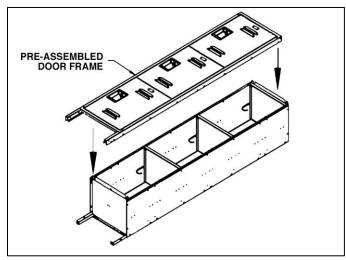
**Step 5:** Tighten all fasteners checking for squareness of the locker while tightening. Attach optional sloping hood, end bases or front bases (see pages 4 and 5).
