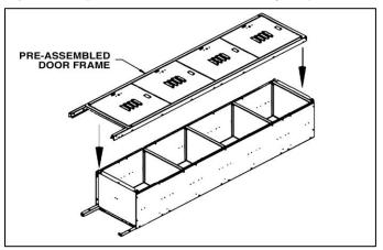
**Step 5:** Tighten all fasteners checking for squareness of the locker while tightening. Attach optional sloping hood, end bases or front base (see pages 4 and 5).
