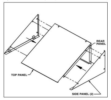
Step 3: Attach the sloping hood to the top of the locker with slotted #8 - 32 screws (provided).
