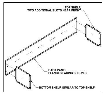
**Step 2:** Turn the back panel on its back with the shelves pointing upward. Attach the first side panel, the left rear leg, and three compartment dividers to the assembly from Step 1.
