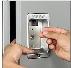
With one hand, hold the case assembly in place. With the other hand, insert the screws through the front of the hasp, continuing through the holes of the case assembly.
