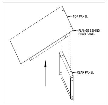
Step 2: Attach the side panels to the top panel and rear panel. Sloping hood assembly is now complete.
