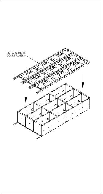
Step 9: Tighten all fasteners, ensuring the locker remains square during the process. If desired, attach optional sloping hood, end bases, or front base (see pages 4 and 5).
