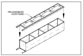
Step 5: Tighten all fasteners, ensuring the locker remains square during the process. If desired, attach optional sloping hood, end bases, or front base (see pages 4 and 5).
