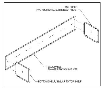
Step 2: Turn the back panel onto its back with the shelves pointing upward. Attach the first side panel, the left rear leg, and three compartment dividers to the assembly from Step 1.
