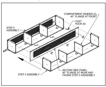
**Step 5:** Attach a third top shelf, a third bottom shelf, and three additional coat hooks to a third back panel (as in Steps 1 and 3).
