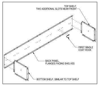
Step 2: Turn the back panel on its back with the shelves pointing upward. Attach the first side panel, the left rear leg, and the hat shelf to the assembly from Step 1. On 15" deep lockers attach the double coat hook to the bottom of the hat shelf and attach a second single coat hook to the first side panel. On 18" deep lockers omit the double coat hook and substitute a single coat hook with a double bend (not shown) instead of the second single coat hook (this will accommodate the coat rod).
