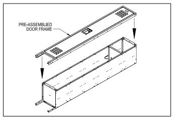
**Step 5:** Tighten all fasteners checking for squareness of the locker while tightening. Attach optional sloping hood, end bases or front bases (see pages 4 and 5).
