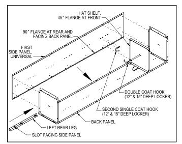
**Step 3:** Attach the second side panel and the right rear leg to the assembly of Step 2. On 15" deep lockers attach a third single coat hook. On 18" deep lockers substitute a single coat hook with a double bend for the third single coat hook and install the coat rod as shown on page 3. The locker chassis is now complete.
