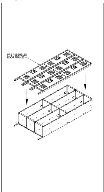
**Step 9:** Tighten all fasteners checking for squareness of the locker while tightening. Attach optional sloping hoods, end bases or front bases (see pages 4 and 5).
