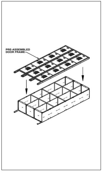
**Step 9:** Tighten all fasteners checking for squareness of the locker while tightening. Attach optional sloping hoods, end bases or front bases (see pages 4 and 5).
