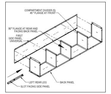
**Step 3:** Attach the second side panel and the right rear leg to the assembly of Step 2. The locker chassis is now complete.
