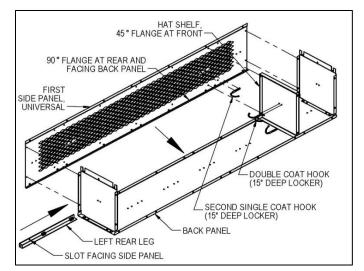
**Step 3:** Attach the second side panel and the right rear leg to the assembly of Step 2. On 15" deep lockers attach a third single coat hook. On 18" deep lockers substitute a single coat hook with a double bend for the third single coat hook and install the coat rod as shown on page 3. The locker chassis is now complete.
