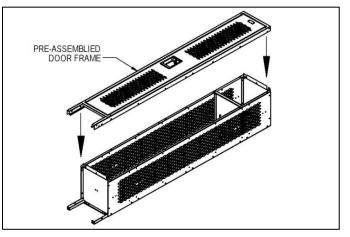
**Step 5:** Tighten all fasteners checking for squareness of the locker while tightening. Attach optional sloping hood, end bases or front base (see pages 4 and 5).
