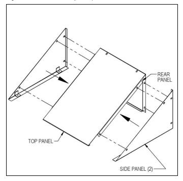
Step 3: Attach the sloping hood to the top of the locker with slotted #8 - 32 screws (provided).
