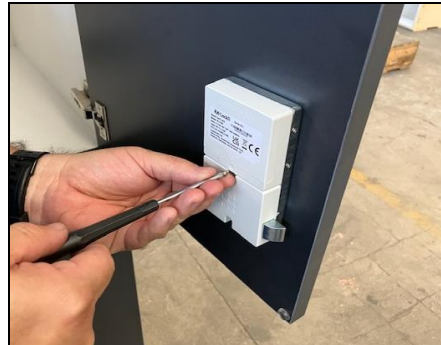
Step 12: Reinstall the Battery Cover Reinstall the battery cover using a PH1 Phillips screwdriver. Confirm all the components are properly installed.
