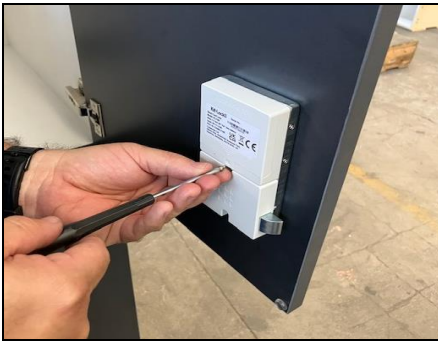
Step 2: Remove the Battery Cover
