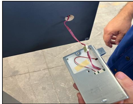
Step 6: Disconnect the Wiring from Battery
