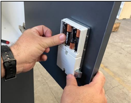
Step 11: Install the Batteries Reinsert the batteries and verify that the electronic lock powers on correctly.
