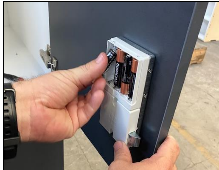
Step 3: Remove the Batteries
