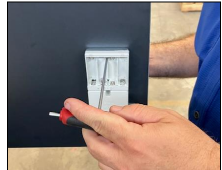
Step 4: Remove the Internal Top Screw
