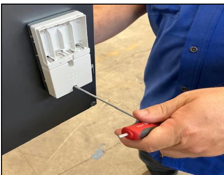
Step 5: Remove the External Bottom Screw
