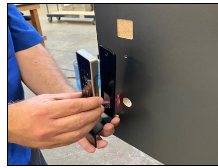
Step 7: Install the ADA Pull Handle
