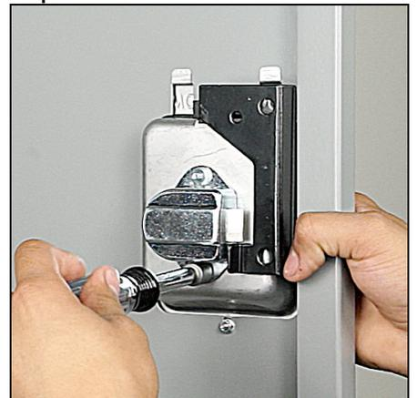
Place locking nuts on screw bolts and tighten. Lock is now ready to operate. **WARNING:** If electric socket wrench is used, do not exert excessive pressure.
