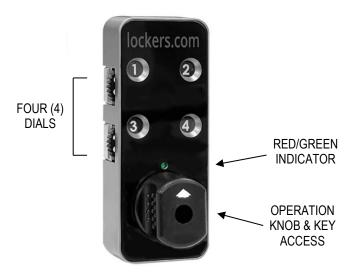
The lock features (4) number dials for setting a 4-digit user combination. When the lock is in the "closed position", the arrow on the operation knob will be in the 9-oclock position and a red indicator appears in a window above the operation knob. When the lock is in the (open position), the arrow on the operation knob will be in the 12-o'clock position and a green indicator appears in the window above the operation knob.
