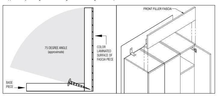
Align front of fascia with front edge of compartment (not the front edge of the door). Install the front filler fascia by fastening it to the lockers by installing screws from inside the lockers into the base of the front filler fascia. #8 x 1-1/4" long screws are provided for the installation.
