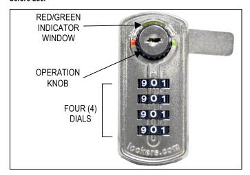
The lock has a four (4) digit combination setting. When the lock is locked (closed), a red indicator appears in a window above the operation knob. When the lock is unlocked (open), a green indicator appears in the window.
