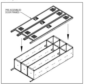
**Step 9:** Tighten all fasteners checking for squareness of the locker while tightening. Attach optional sloping hoods, end bases or front bases (see pages 4 and 5).
