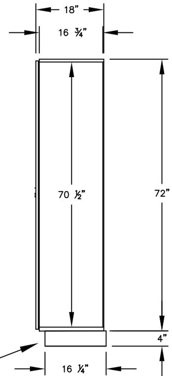
(BASES ARE MADE OF INDUSTRIAL GRADE PARTICLEBOARD AND ARE COVERED IN A DURABLE BLACK LAMINATE. PLEASE SET BASE TO ALLOW 5/8" BETWEEN THE BACK OF THE LOCKER AND THE WALL FOR AIR VENTILATION.)
