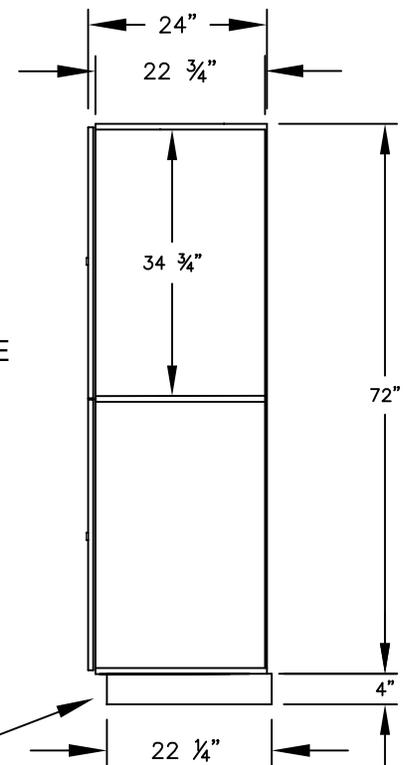
(BASES ARE MADE OF INDUSTRIAL GRADE PARTICLEBOARD AND ARE COVERED IN A DURABLE BLACK LAMINATE. PLEASE SET BASE TO ALLOW 5/8" BETWEEN THE BACK OF THE LOCKER AND THE WALL FOR AIR VENTILATION.)
