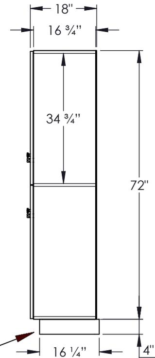
(BASES ARE MADE OF INDUSTRIAL GRADE PARTICLEBOARD AND ARE COVERED IN A DURABLE BLACK LAMINATE. PLEASE SET BASE TO ALLOW 5/8" BETWEEN THE BACK OF THE LOCKER AND THE WALL FOR AIR VENTILATION.)
