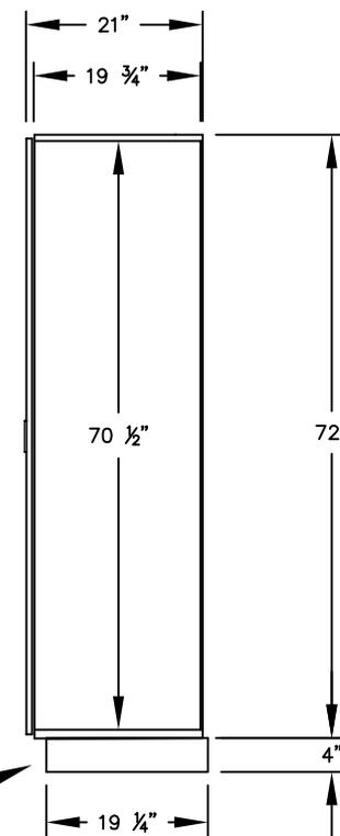
(BASES ARE MADE OF INDUSTRIAL GRADE PARTICLEBOARD AND ARE COVERED IN A DURABLE BLACK LAMINATE. PLEASE SET BASE TO ALLOW 5/8" BETWEEN THE BACK OF THE LOCKER AND THE WALL FOR AIR VENTILATION.)
